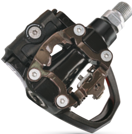
SIDE B: EPS-M (Compatible with Shimano SPD).
